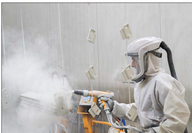
Powder coating with a spray gun
