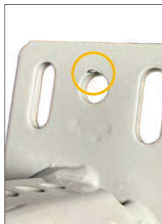
Suspension point after coating
